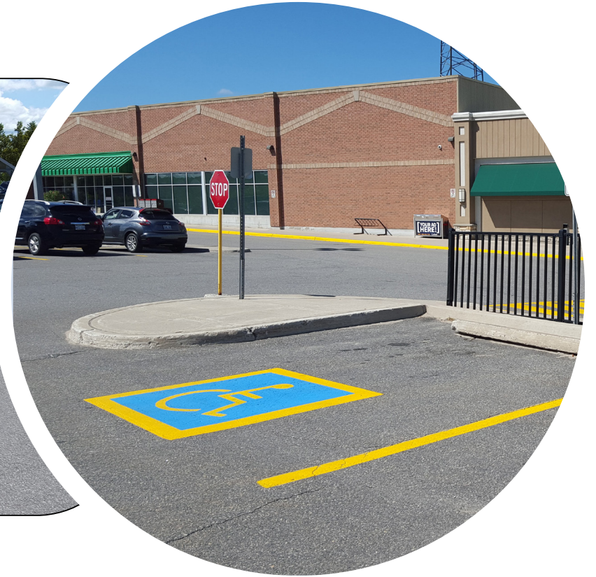
Some of the challenges with the accessible parking spaces in the downtown, and in newer developments, is that they are not connected to a safe route of travel; there are missing curb cuts; they are not located in the optimal locations. These are all easy things to address.
