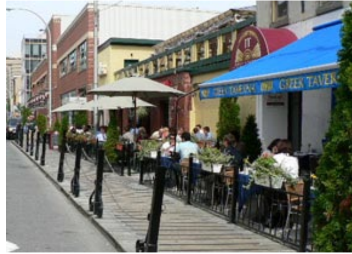
In these two images, the sidewalk has been re-directed around the patio space, into the street parking area. Note the various barriers and use of planters.
